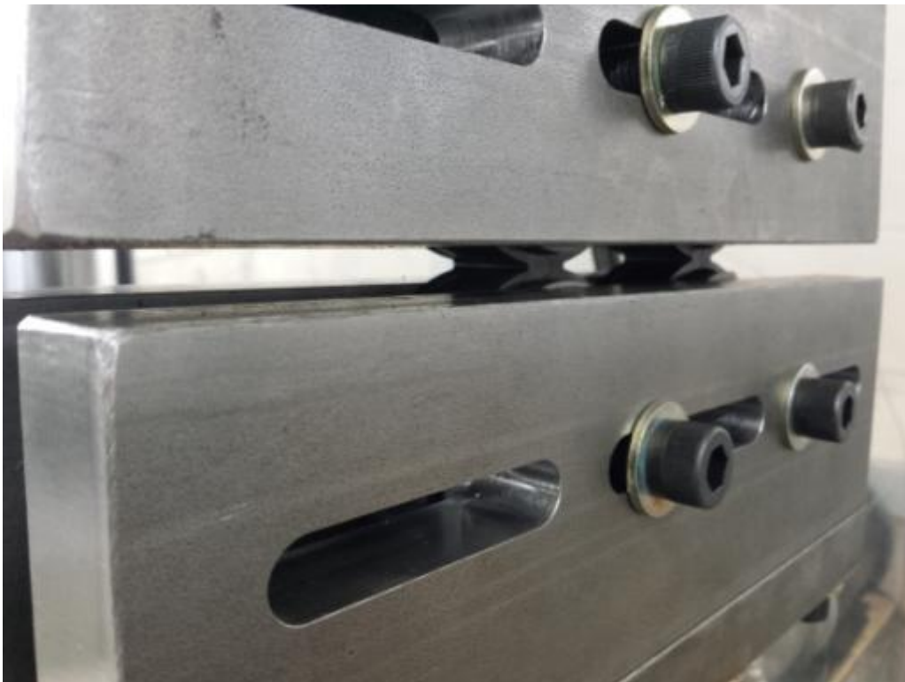
Figure 6 – A close up photograph of the test setup for a 4 cell bond tension test.
