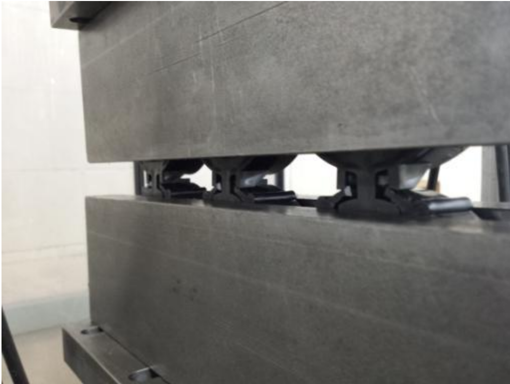
Figure 5 – A close up photograph of the back side of the test setup for a triple tab pull apart.
